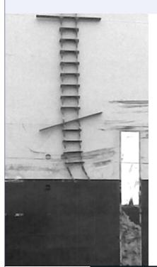
◆ This ship has a freeboard where the distance from sea level to the point of access to, or egress from the ship exceeds 9 metres as indicated by the IMO pilot freeboard mark on the ship's side.
